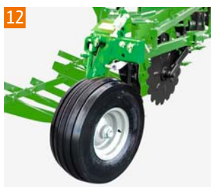
Wheel Ø 680 mm air-filled tyre x 250 mm wide Suitable for: XMS/XS (not for 6 furrow or 5 furrow S and/or V ploughs)
