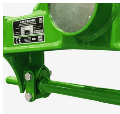
Turnover cylinder with interconnected pivot mechanism
