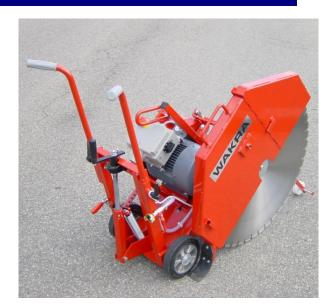
A very compact floor saw with electric engine, mounted on quick disconnection plates. The working feed is handled by pushing. Blade admission left and right side, up to max. 800mm! Blade lowering by crank mechanism. Thanks to water supply through cutting shaft and flanges, an optimal blade cooling is guaranteed. Depth adjustment indicator, crane suspension.
