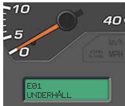
EMMS (Equipment Management and Monitoring System)
