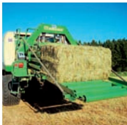
BiG Pack 1270 (2'x4') (X-Cut): This machine is used in conditions because of its chamber dimensions of 120 cm (3'11") height and 70 cm (2'4") width. Six Single or Double Knotters provide for well-shaped baling in straw, hay and silage.
