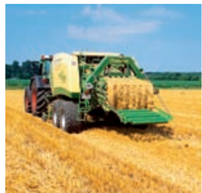
BiG Pack 1270 (X-Cut/MultiBale): With this version you can pack up to nine small bales in one large bale. Your benefits: The large bales can be cleared quickly from the field and the small bales can be easily distributed.
