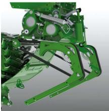
Using the grain conditioner In this position, the crop flows through the corn conditioner. This way, the conditioner can subject the kernels to intensive treatment to make the nutrients available.
