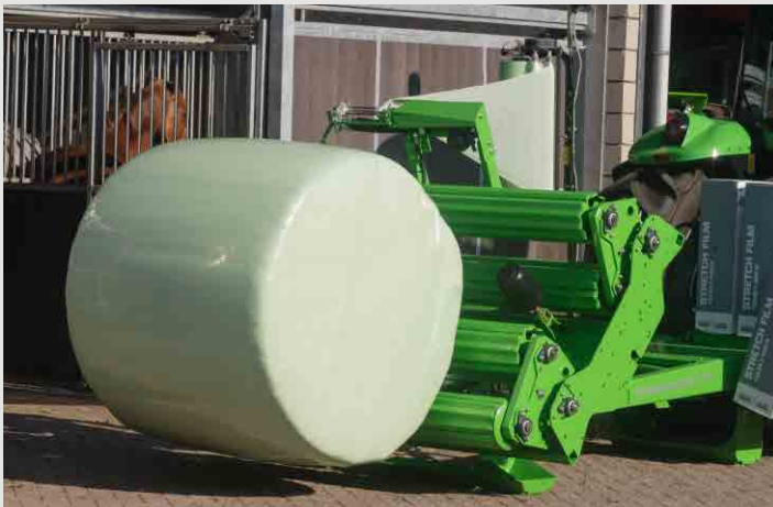
THE LOW TABLE HEIGHT ALLOWS THE BALE TO BE GENTLY TIPPED OFF TO PREVENT FILM DAMAGE
