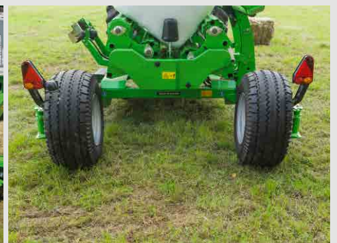
FOR ROAD TRANSPORT THE WHEELS CAN BE FOLDED INWARDS TO REDUCE THE TRANSPORT WIDTH. HYDRAULIC FOLDING IS OPTIONAL.
