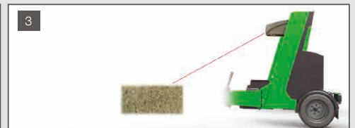
LASER SENSOR HAS DETECTED THE EDGE OF THE BALE. BALE LENGTH MEASUREMENT IS STARTING BY COUNTING PULSES ON WHEEL SENSOR. LOADING ARMS MOVE TO PRE-LOAD POSITION (BASED ON PRE-DEFINED BALE WIDTH).
