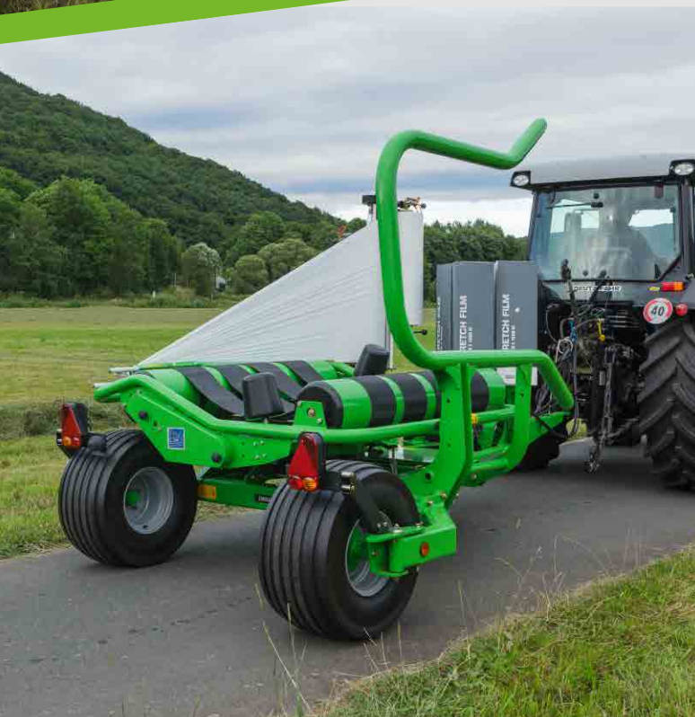
LIMITED TRANSPORT WIDTH DUE TO ADJUSTABLE WHEEL POSITIONS.
