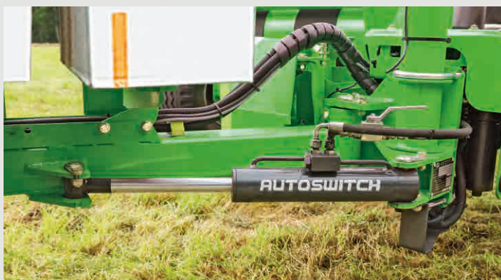
AUTOSWITCH FUNCTION, EASY INTO WORK OR TRANSPORT POSITION
