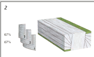
2 THE BALE IS COVERED WITH 3 LAYERS AND 67% OVERLAP
