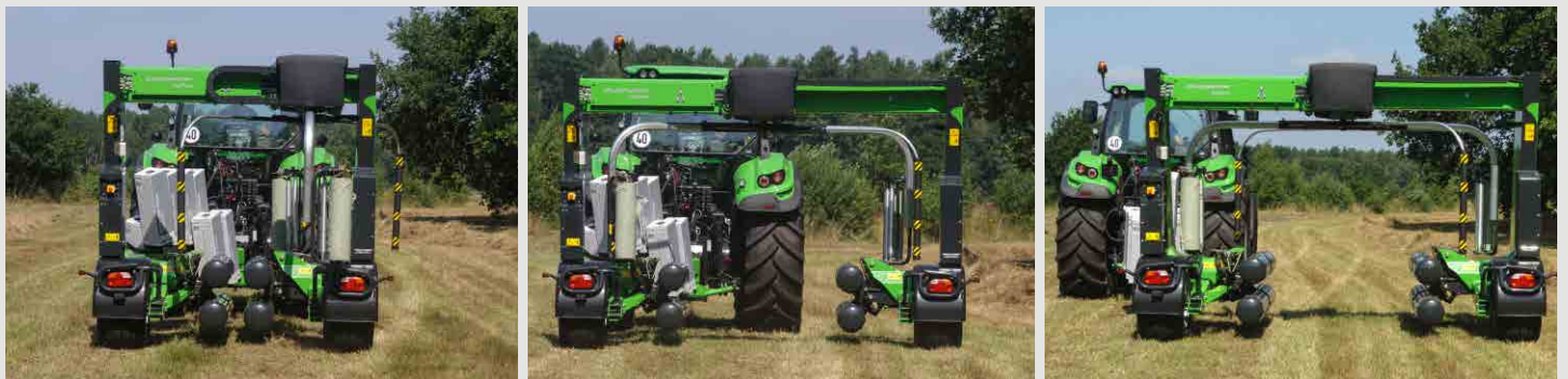
THE WRAPPER FOLDS FROM ITS 2,5 M TRANSPORT POSITION INTO 4 M WIDE FIELD POSITION.
