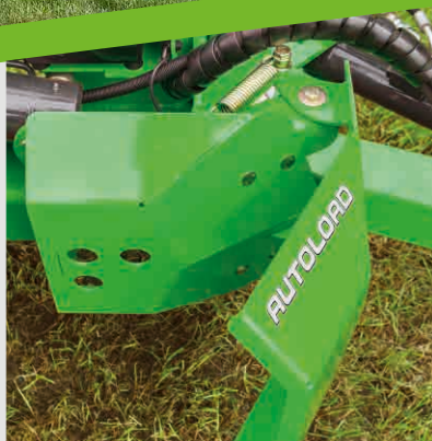
AUTOLOAD, AUTOMATIC BALE PICK-UP SYSTEM
