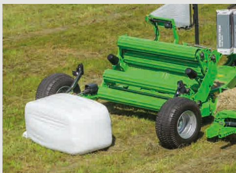
THE LOW TABLE HEIGHT ALLOWS THE BALE TO BE GENTLY TIPPED OFF TO PREVENT FILM DAMAGE.
