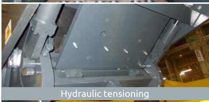
Hydraulic gap adjustment to prevent clogging
