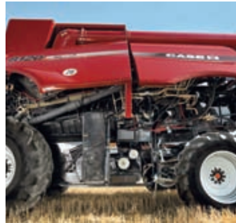
▲ Large side panels. Composite panels open easily to expose the interior of the combine.
