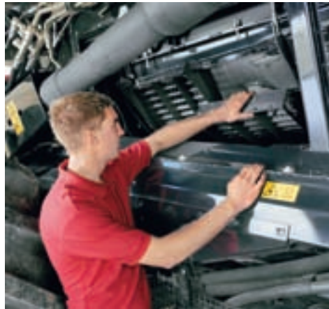
▲ Easy access to concaves and rotor. Cleaning or changing the concaves and rotor rasps has been made easy.
