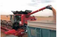
▲ Huge capacity grain tank. Up to 10,500 litre grain tank with electrically controlled quick-folding extensions that don't require tools. The tank is completely closed in the folded down position.
