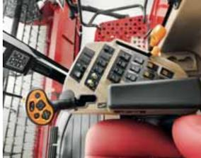
Clear overview with A-post instrument cluster. At-a-glance information on the status of the combine, including engine power, header tilt, residue direction, electrical sieve settings, diagnostics and service reminders.
