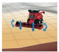
▲ Perfect ground hugging. The Terrain Tracker header control system keeps the header parallel to the ground in undulating conditions.
