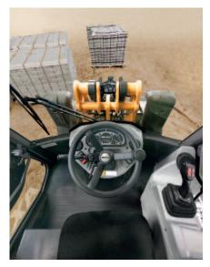
Optimum front and rear view due to monoboom and compact rear end
