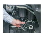
The engine oil dipstick is easy to reach even when a front loader is fitted
