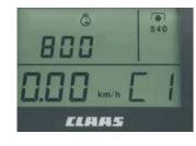
The current gear is indicated on the instrument panel at all times, and also in the A-pillar on CIS+
