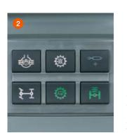
Control panel for main functions: differential lock, four-wheel drive, road or field mode, hydraulic pump aggregation and activate front axle suspension
