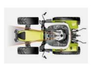
The tapered bonnet provides optimum visibility as it becomes narrower towards the bottom and towards the driver
