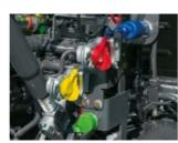
Air brakes and hydraulic brakes are also available in combination
