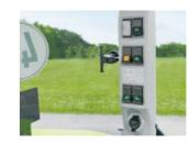
Switches for the work lights are conveniently positioned on the left-hand B-pillar
