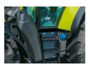
Filler necks for 17 or 22 I urea solution and 140 or 190 I fuel by the cab access
