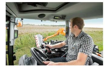
5-pillar cab with large continuous and shatter-proof right-hand side window made from polycarbonate is ideal for municipal verge mowing
