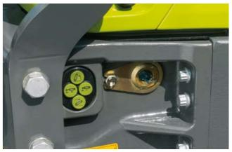
With electronic spool valves, the front linkage and additional spool valve can controlled externally
