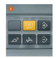
Control panel for additional functions: safety switch for front loader attachment locking, activate automatic PTO engagement/ disengagement, activate dynamic steering, fine adjustment of engine speed memories
