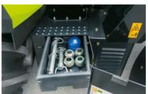
The battery and a storage compartment for tools are located in an accessible position to the right of the steps
