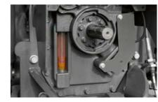
Hydraulic and transmission oil levels are easily checked using the sight glass next to the PTO
