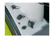
ISOBUS connections in the cab and at the rear
