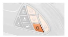
The switch to activate the auto-shift function is within easy reach on the multipad
