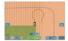
With AUTO TURN the tractor turns automatically at the headland
