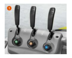
Controls for both mechanical and electronic spool valves are conveniently located on the side console
