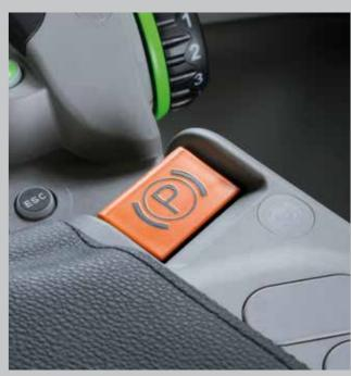
$TTV\ models-EPB\ replaces\ the\ mechanical\ handbrake\ lever\ and\ is\ operated\ via\ an electric\ push-button\ control\ on\ the\ armrest\ console.$
