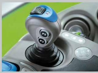
Hydraulic valves can be managed through proportional and programmable controls in terms of time and quantity. The electronic joystick can be programmed to use the front loader, whereas other tractor functions can be operated using the thumbwheel
