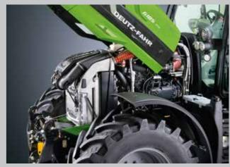
Highly efficient and compact cooling system with intercooler, engine, transmission fuel cooler, and air conditioning condenser.
