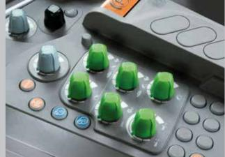
Fine-tuning front (TTV only) and rear lift control can be operated through the potentiometer on the armrest.
