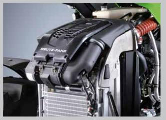
PowerCore technology air filter: 20% higher air flow capacity than comparable standard filters.
