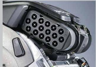
Precleaning system of the air intake filter: spiral cyclone tubes and an aspirate hose removes 95% of the dust before entering the primary filter.
