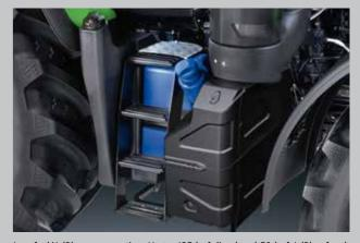
Low fuel/AdBlue consumption. Up to 435 Lof diesel and 50 Lof AdBlue for the six-cylinder, and up to 225 Lof diesel and 28 Lof AdBlue for the four-cylinder facilitate longer working days.
