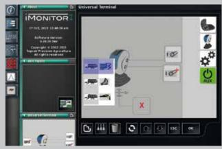
ISOBUS integration. Equipment functions controlled via defined tractor key
