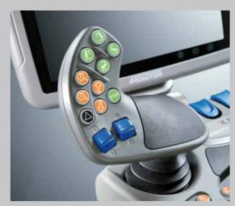
By simply pressing two buttons on the MaxCom multifunctional lever, the driver can recall four different speed settings whether in the field or on the road and maintain a constant speed for optimum results.
