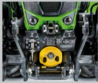
New front lift position control (TTV models) with maximum lifting power of 5,480 kg.
