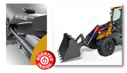
Increase of lifting power due to compensation cylinder by 17%
