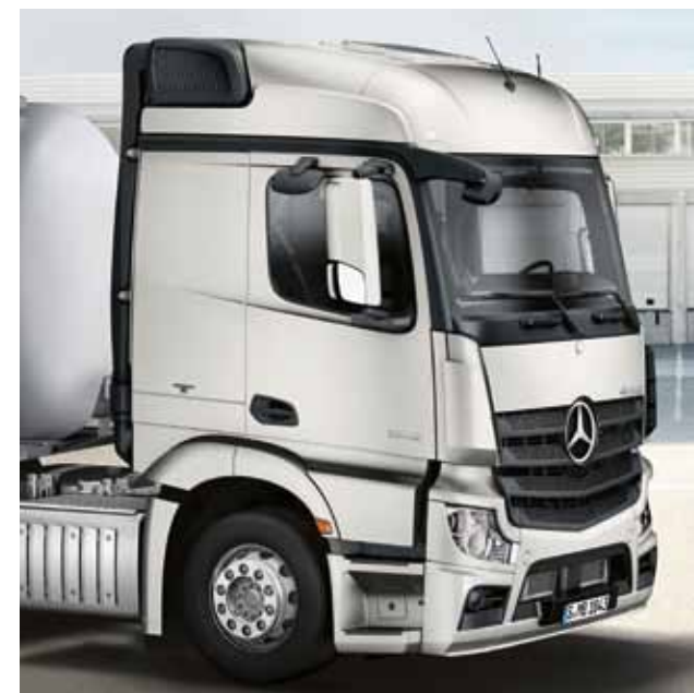
Cab sidewall without locker door. Less unladen weight, more payload. The closed cab wall on the right-hand side results in a weight saving of five kilograms.
