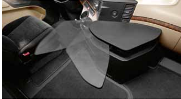
Convenient and space-saving. The height-adjustable folding table finished in artificial leather is ideal for meals, for working on a laptop computer or for use as a convenient stowage tray.
