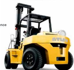
Reliable, stable and safe counterbalance truck with fuel saving engine technology. Convenient boarding, excellent all-around visibility and a powerful design made for rough handling. Lift capacity 5000/6000/7000 kg Lift heights up to 6.0 metres
