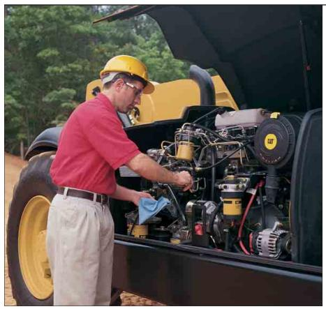
Access. All Cat Telehandler service points, including the combined transmission/hydraulic oil filter, are readily accessible and major components are easy to reach at ground level due to the overall machine design. A cab mounted service point allows access to the fuel fill, hydraulic oil fill, washer bottle, fuse box and cab air filter for daily checks.
