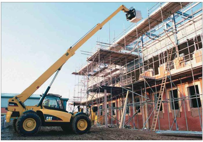
**Lift Height.** The TH460B can effectively and quickly place bricks, roofing materials and trusses to a maximum height of 13 500 mm.
