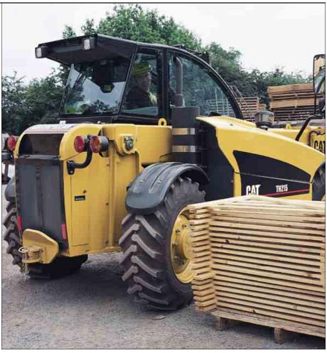
**Steering Modes.** The compact telehandlers offer three steering modes, (circle, two wheel and crab steer) to allow an operator to easily position the machine in small, confined areas. Steering modes are selected by using the steering mode switch in the operator's compartment. An indicator light in the cab illuminates when the wheels are properly aligned.
