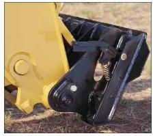
**Manual Coupler.** The TH215 utilizes a manual quick coupler using the same interface as the Caterpillar Skid Steer Loader.
