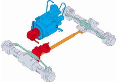
**Engine.** The TH215 is powered by the well-proven Caterpillar 3054B-DI Naturally Aspirated diesel engine. This provides high fuel efficiency and excellent reliability developing full torque at lower revs compared to other engines.
