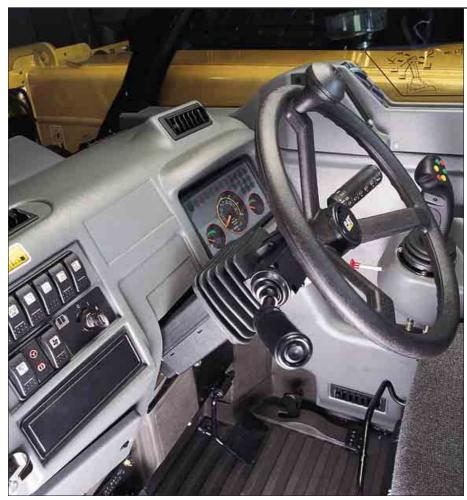
**Enclosed Cab.** The TH215 is equipped with an enclosed cab allowing the operator to work comfortably, with air conditioning available as an option. The cab structure has been designed and certified to provide falling object and rollover protection (FOPS/ROPS).
