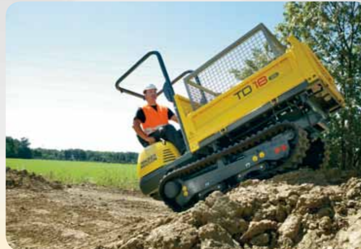
The Euro pallet dimensions of the 3 sided tipping skip greatly extends the areas of deployment of the TD18. This gives it additional functions as a specialist for transport tasks in difficult terrain.
