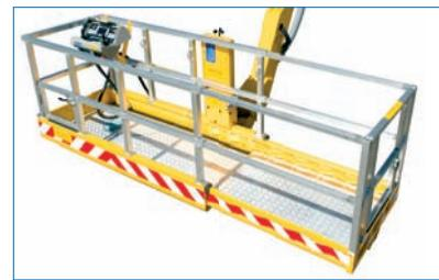
Cage slewing 90 degrees. Hydraulically extendable cage available as an option.
