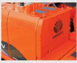
Large fuel tank The fuel tank with 280 liter capacity has been mounted to reduce filling up interval.
