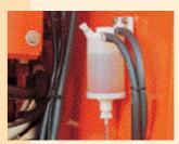
Water separator The transparent glass water separator is mounted at a location easily accessible from the ground allowing easy maintenance of the fuel system.
