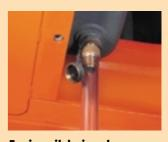
**Engine oil drain valve** The engine oil drain valve with quick coupler provides fast and enviromentally sound serviceability.
