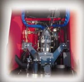
You can reach the hydrostatic transmission and the hydraulic system easily and inspect them completely thanks to the cabin hydraulic tilting system.
