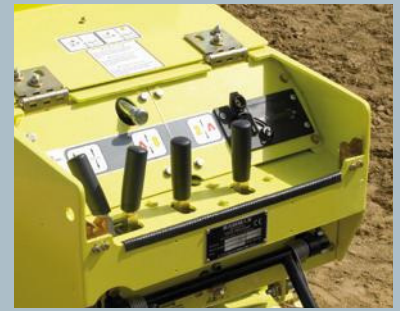
Modern and clearly arranged cockpit with failure diagnostic system and function control
