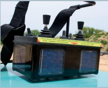
IR transmitter with solar panels
