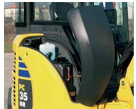
Front bonnet: fuel tank refilling
