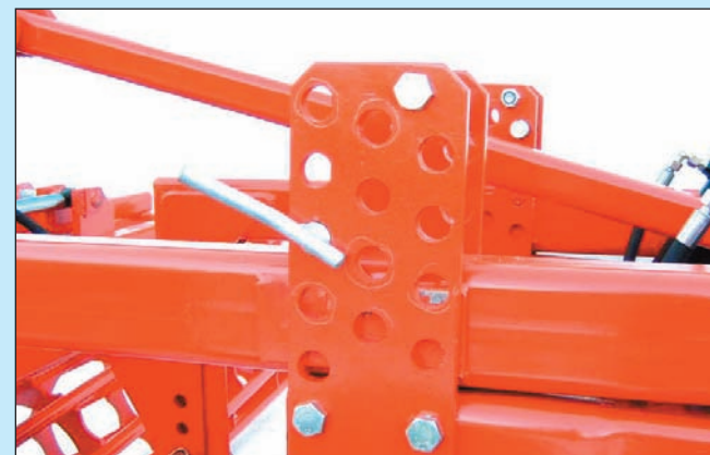
Working depth is adjusted via a perforated rail and peg bolts for the "Leader". The transport wheels turn freely when working.
