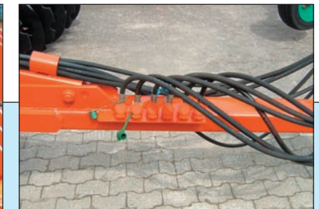
Clean storage of hoses when not in use.
