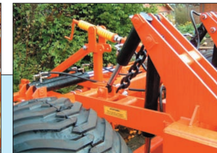
Hydraulic depth adjustment via rear roller.
