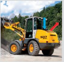
Cooling air is drawn in from the 'cleanest' zone directly behind the rear window
