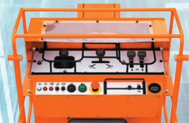
Operating panel designed for safety (Upper control panel)
