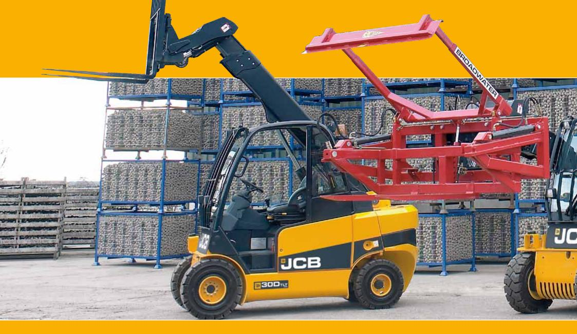
First take the small footprint of an industrial counterbalanced lift truck. Then add the telescopic boom of a telescopic handler. Design-in a fully enclosed hydrostatic drive system. Then finish off with a hydraulic quick-disconnect carriage for forks or shovel.
