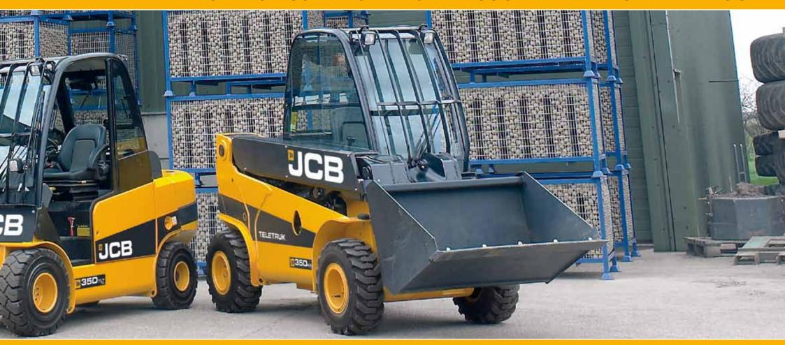
versatile small counterbalanced lift truck. The JCB Teletruk is not just another lift truck. The range covers the most popular 2.5t – 3.5t capacity bands; diesel-powered two-wheel drive or four-wheel-drive, and two-wheel drive gas models.
