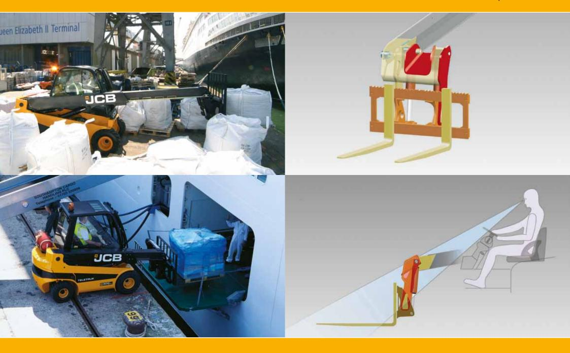
The JCB Teletruk range comprises ten compact models with diesel powered fully-enclosed hydrostatic drivelines in two and four-wheel-drive, and two
