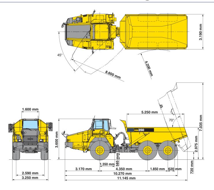
All measurements with tyres 26.5 R25; if equipped with tyres 800/65 R29: Overall height 3.670 mm, overall width 3.500 mm, tread 2.710 mm
