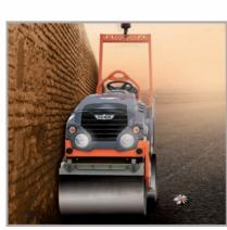
HD 10C VV - Articulated tandem roller with two vibratory drums
