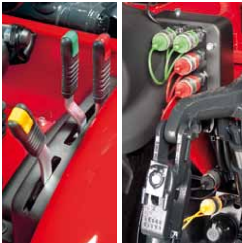
Hydraulic system with 3 manifolds: 1 double-acting, 1 double-acting with floating position and stop lever, 1 single-acting + oil return tap. Total: 6 rear quick-couplers.
