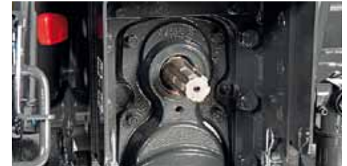
Two speed PTO: 540 rpm, 540 E (750 rpm) and synchronized with gear speeds. The PTO shaft of the ASAE 1 3/8 type is the same for all speeds.
