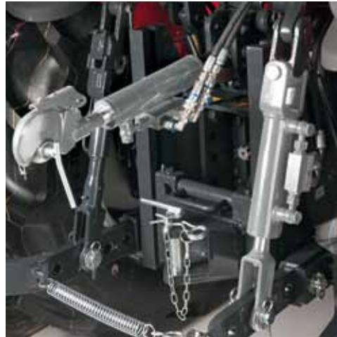
Vertical hydraulic tie-rod and 3-point hitch* allow adjustments to be made from the driver's seat.
