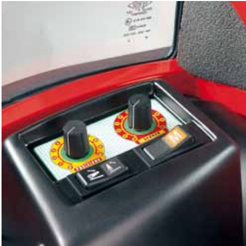
Buttons for lifting position with memory*: two potentiometers for adjusting position, draft, and hydraulic lift block for road transport.
