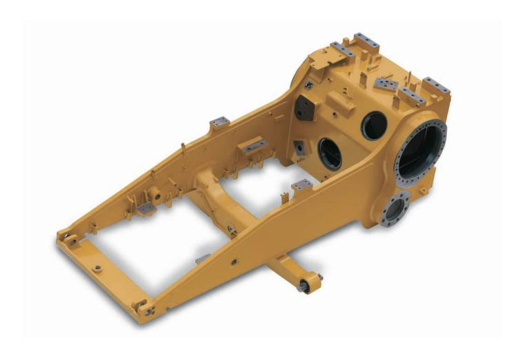
**Frame and Castings.** The D6T frame is built to absorb high impact shock loads and twisting forces. The frame has a reinforced saddle and a welded front cross-member that add strength to the frame to better handle lateral and twisting forces. Steel castings augment the strength of the main case.
