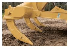
**Multi-Shank Ripper.** The multi-shank parallelogram style ripper offers the choice of one, two or three shanks depending on job conditions. Curved or straight ripper shanks are available.
