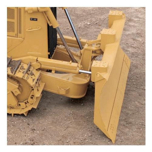
**Cat® Blades.** All blades feature a strong box-section design that resists twisting and cracking. Blades are made of Cat DH-2<sup>TM</sup> steel that has high tensile strength and stands up to the most severe applications. Heavy moldboard construction and hardened bolt-on cutting edges and end bits add strength and durability.
