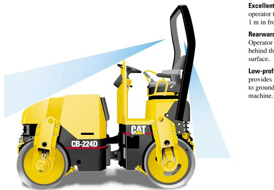
**Excellent forward visibility** allows the operator to see objects 0.58 m high and 1 m in front of the machine.
