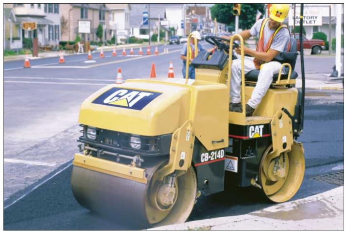
The CB-214D, CB-224D and CB-225D are versatile machines that can be used as the only compactor on small sized jobs or on larger jobs as a support roller for high-production compactors. As a support roller, they work well for turning lanes, crossovers, shoulders and other similar sized jobs.
