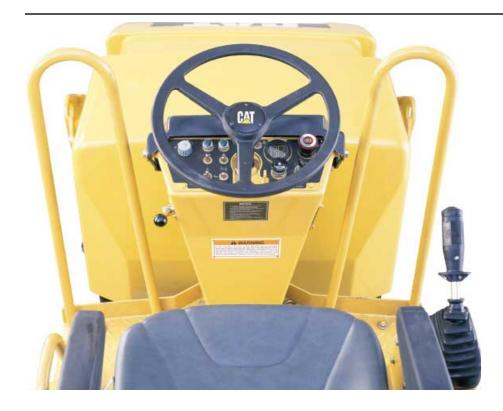
**Single-lever control** provides simplified operation, making the machines a perfect fit for inexperienced operators.
