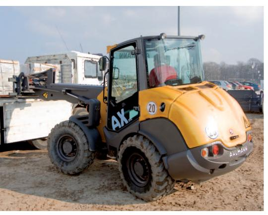
Due to the ASAP-monoboom, the Ahlmann AX features high breakout forces. Its Z-kinematics allow for perfect parallel guidance of attachments. This results in a high degree of safety, in particular when loading pallets. Fast tipping cycles and an excellent view on the attachments make daily work even more efficient.
