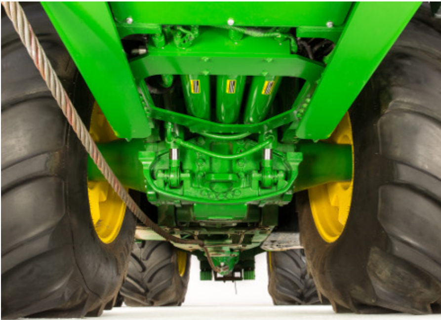
9R 640 equipped with HydraCushion suspension
