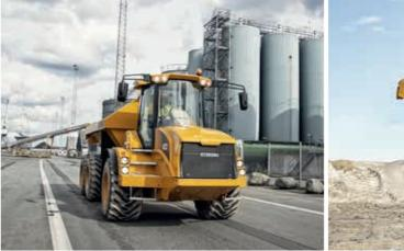
The intelligent transmission effectively translates the engine's 314 hp and 1288 Nm of torque into the maximum tractive effort. Moreover, the advanced transmission shifting system guarantees a smooth gear shift, that prevents the wheels from slipping and continues to provide maximum torque and traction.
