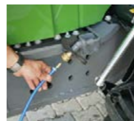
□ There is a compressed air connection at the machine front to blow out the air from the radiator.
