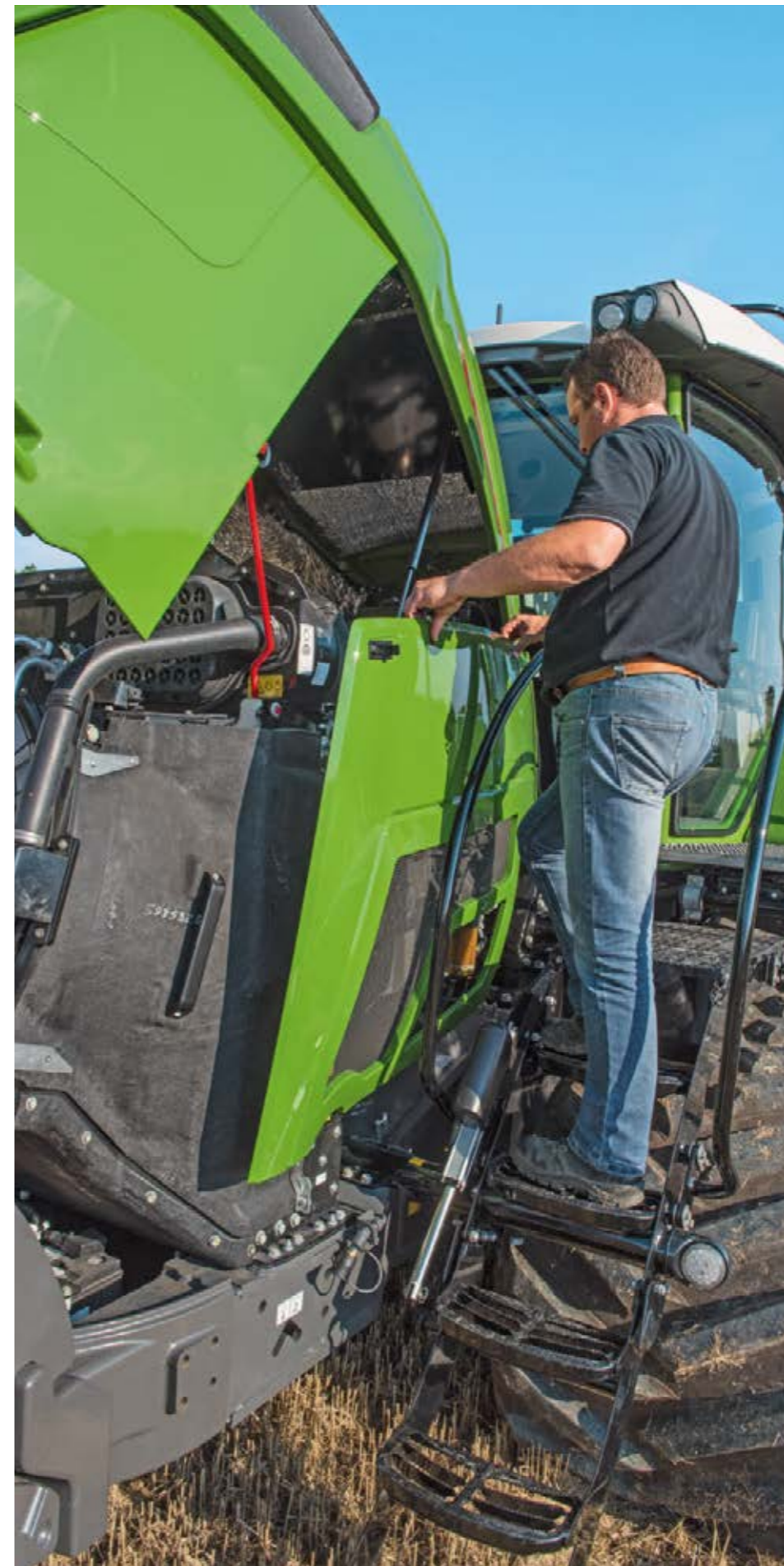
There is sufficient room for maintenance thanks to the large one-piece cover. You can comfortably reach the air filter from the ladder.
