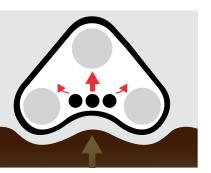
Alternative design: With 3 mid-rollers, vibration is transferred directly upwards into the drive sprocket and axle. This results in an uncomfortable ride.
