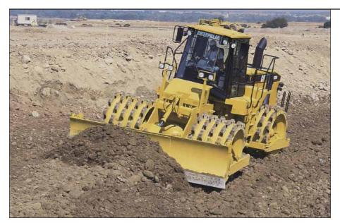
**Wheel Tips.** There are 13 tips per row and 65 tips per wheel for excellent compaction.
