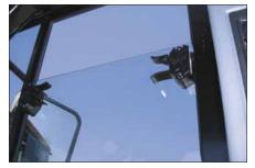
**Optional Sliding Cab Windows.**Are located in the right and left doors to provide access to outside air without opening the door.
