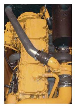
**Caterpillar 3406E Engine.** Is a six-cylinder, turbocharged, air-to-air aftercooled (ATAAC), Electronic Unit Injection (EUI) engine and one of the most developed and proven engines offered by Caterpillar. It has a strong reputation for reliability, durability and performance.
