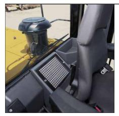
**Air Conditioning.** Is standard and uses blended air for immediate temperature changes, clears windows easily and improves operator comfort. The cooling system is located behind the operator's seat and uses R134a refrigerant.
