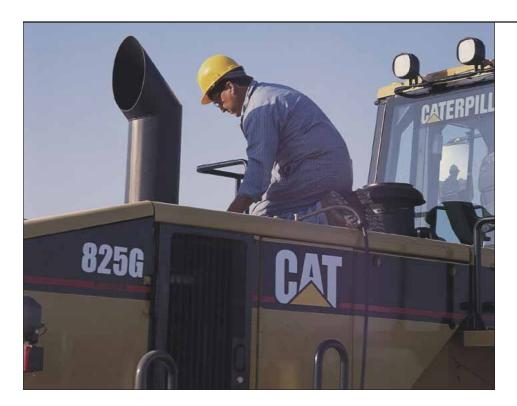
**Engine Access.** New engine enclosure replaces a non-metallic hood assembly which increases durability in tough applications where soil conditions are less than optimum.
