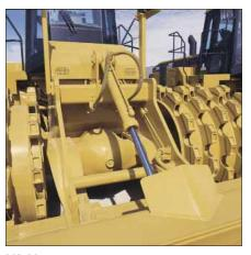
**Lift Lines.** Are located in a high location above the cylinder yoke where damage is less likely to occur.
