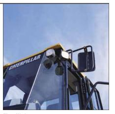
**Floodlights.** Located on the 825G Series II exterior are super damp and will last up to seven times longer than previous lights.
