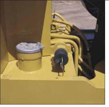
Fast Fuel Fill. Used during peak periods when high production is needed and little down time can be afforded for fueling. Fuel is pumped into the tank through a filling nozzle at rates up to 378.5 liters per minute. As fuel enters the tank, air is forced out through an open vent. When the tank is full, the vent closes and the filling nozzle automatically shuts off.
