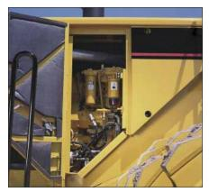
Service Access. Scheduled maintenance points are well within reach. An air filter service indicator is visible from the cab or platform, with the air filter accessible from the left platform and the engine oil filter from the right platform. A remote grease fitting is provided to lubricate the lift cylinder yoke. Removable treadplates in the platform give access to less commonly serviced components.
