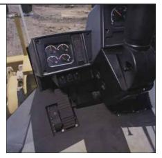
**Decelerator Pedal.** Provides engine deceleration for the first 50 percent of travel and then the brake engages. This left pedal enables the operator to slow down when the throttle lock is engaged and to return to throttle lock without pressing a button.
