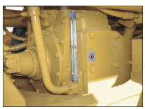
**Transmission Oil Fill Tube.** Is located beneath the platform area and the transmission oil dipstick has a sight gauge next to the fill tube for easy maintenance.
