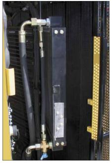
**Hinged Hydraulic Oil Cooler.**Can be swung open 30 degrees without special tools.
