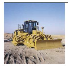
**Blade Package.** Consists of the blade, push-arms, trunnion mounting, dozer-length skid plate with replaceable wear plates, reversible cutting edges, selfsharpening end bits, hydraulic lines guard and hydraulic lift cylinders.
