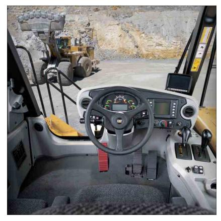
**Operator Controls.** Easy to reach turn signal, high beam, intermittent windshield wiper and windshield washer controls are located on the left side of the steering column, and are designed for optimum efficiency and comfort.
