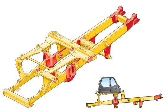
**Box-Section Design.** The 775F frame uses a box-section design, incorporating two forgings and 19 castings in high-stress areas with deep penetrating and continuous wrap-around welds to resist damage from twisting loads without adding extra weight.
