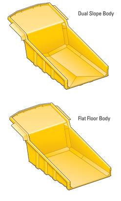
**Body Selection.** Selection of the right body system depends on material, haul road and loading conditions. The better the match of body to application, the greater the efficiency. Cat dealers can help select the right body system for site-specific applications.
