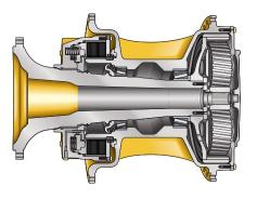
**Long Life.** An oil film prevents direct contact between the discs. This design absorbs the braking forces by shearing the oil molecules and carrying heat away to extend brake life.
