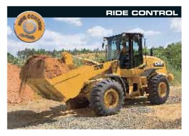
The ergonomically designed Case wheel loaders can be specified with Ride Control, a system that allows the lift arms to float when the machine is moving, preventing bounce in the cab and at the wheels. Ride Control allows the operator to drive at higher speeds during load and carry operations, offering excellent load retention and reducing fatigue for the operator.
