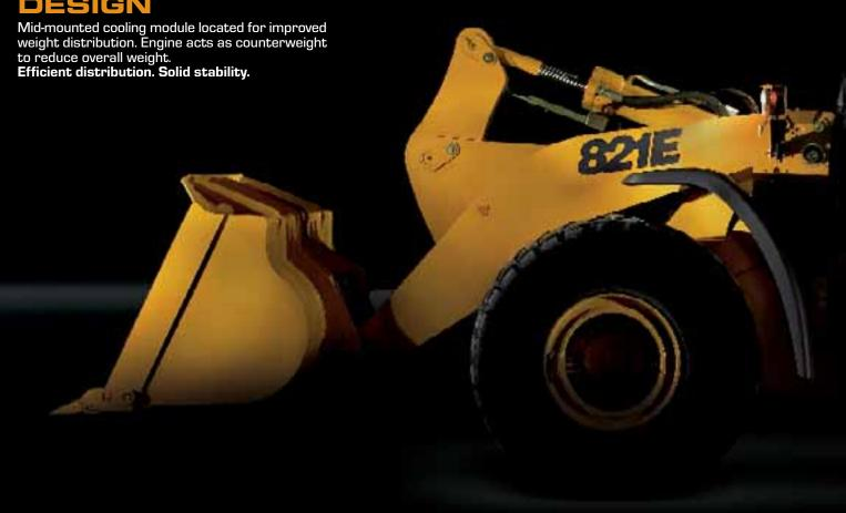
Mid-mounted cooling module ensures constant temperature for increased component life. Automatic reversible fan keeps radiator cores clean, reducing downtime.
