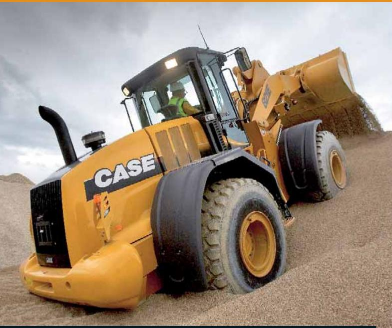
Engine Horsepower Operating weight (max.) Bucket capacity **721E** 137 kW/183 hp 14500 kg 2.40 - 2.70 m<sup>3</sup> **721EXT** 137 kW/183 hp 14650 kg 2.40 - 2.70 m<sup>3</sup> **721EXR** 137 kW/183 hp 15071 kg 2.30 - 2.70 m<sup>3</sup> **821E** 159 kW/213 hp 17166 kg 2.80 - 3.30 m<sup>3</sup>
