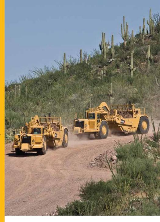
Quick loading, high travel speeds and the ability to load and dump on the run yield fast cycle times, allowing Cat® Wheel Tractor-Scrapers to deliver a high rate of productivity.
