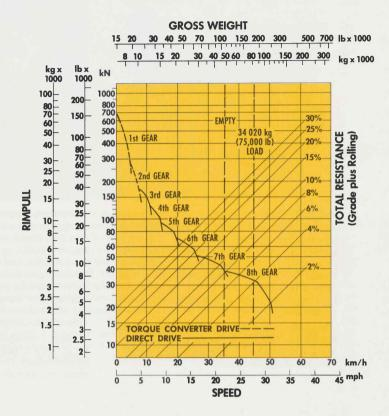
To determine gradeability performance: Read from gross weight down to % of total resistance. (Total resistance equals actual % grade plus 1% for each 20 lb./ton (10 kg/t) of rolling resistance.) From this weight-resistance point, read horizontally to the curve with the highest obtainable speed range, then down to maximum speed. Usable rimpull depends upon traction available and weight on drive wheels.
