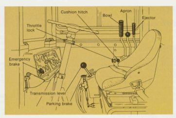
Convenient controls are designed to improve operator efficiency:
