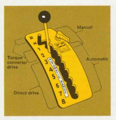
Cat 8-speed transmission combines automatic shifting with high torque multiplication and direct drive efficiency. The transmission shifts up and down automatically between 2nd and the highest selected gear. Reverse and Gears 1 and 2 are torque converter drive for powerful rimpull needed for loading and dumping. Gears 3 through 8 are direct drive for quick acceleration and efficient hauling speeds.
