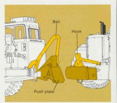
Push-Pull Arrangement allows two 637D Wheel Tractor-Scrapers to assist one another in self-loading. That means no push tractor with operator required . . . no pusher downtime . . . no scraper-pusher mismatch . . . no bunching. You get a balanced, more flexible spread with less investment and fewer machines. The arrangement includes a hydraulically actuated bail and cushion push plate bolted to the front of the tractor and a hook on the rear of the scraper.
