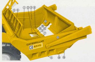
For rock application, a Special Application Scraper is available. Complete bowl is box sectioned for maximum strength, and high-tensile steel is used in high wear and stress areas. Extensive heat treatment is used in bowl bottom plates, side bottom rails, cutting edge support, router bit support and apron front sheet and lip.
