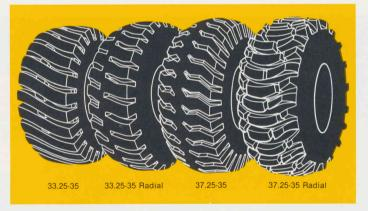
Choose the tires that match your job. Standard 33.25-35, 38 PR (E-3) for good performance on many jobs. Optional radial steel cords in this size are also available. Optional wider tire, 37.25-35, 30 PR (E-3), provides greater load capacity and has a larger contact area to reduce ground pressure and increase flotation. Machines equipped with this tire can negotiate poorer underfoot conditions and travel faster on soft materials.
