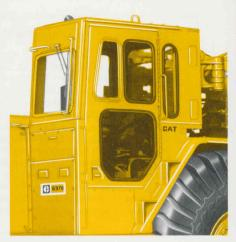
Optional ROPS sound-suppressed cab rests entirely on rubber mountings, with no metal-to-metal contact. Sound is further suppressed with insulated right and back walls, roof headliner and positive seals around windows and door. Seat belt, windshield, windshield wiper are standard. Air conditioner and heater are optional.
