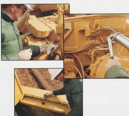
Maintenance platform access — engine oil check and fill, engine coolant level check and fill, front brake reservoir, hydraulic system filter, secondary fuel filter.
