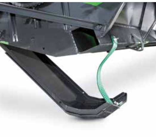
Skids ensure that the header follows the ground contours closely, compensating on the move for every ground undulation.
