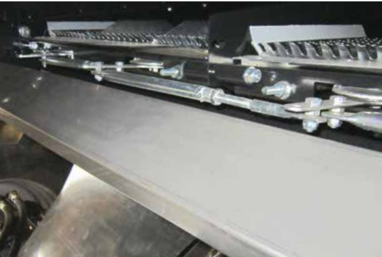
With dual sensors and a control bar along the full length of the sieve box, the sieve performance control system allows precision monitoring of combine productivity
