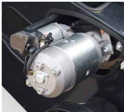
An electrically operated reversing unit is designed to eliminate any overloading of the feed system.
