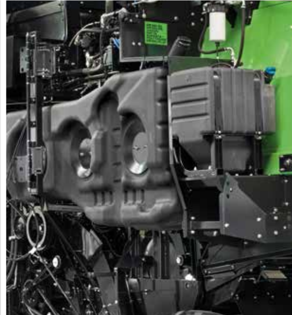
The fuel tanks and AdBlue® tank are made from 10 mm thick polyethylene.
