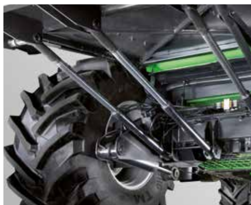
Final drive units rated 25 t enable the machine to work in the most hostile conditions while guaranteeing optimum reliability, and more importantly, maximum operator safety.
