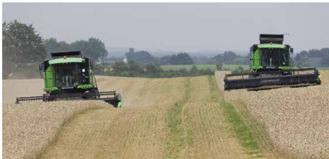
AUTOCONTROL adjusts the lateral and vertical movement of the header with notable precision, so as to maintain a steady cutting height and ensure that laid crops can be harvested to optimum effect, with the cleanest possible cut.
