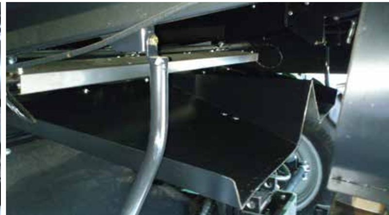
New chaff transfer pan with metal chutes that direct the chaff towards the 4-blade rotors.
