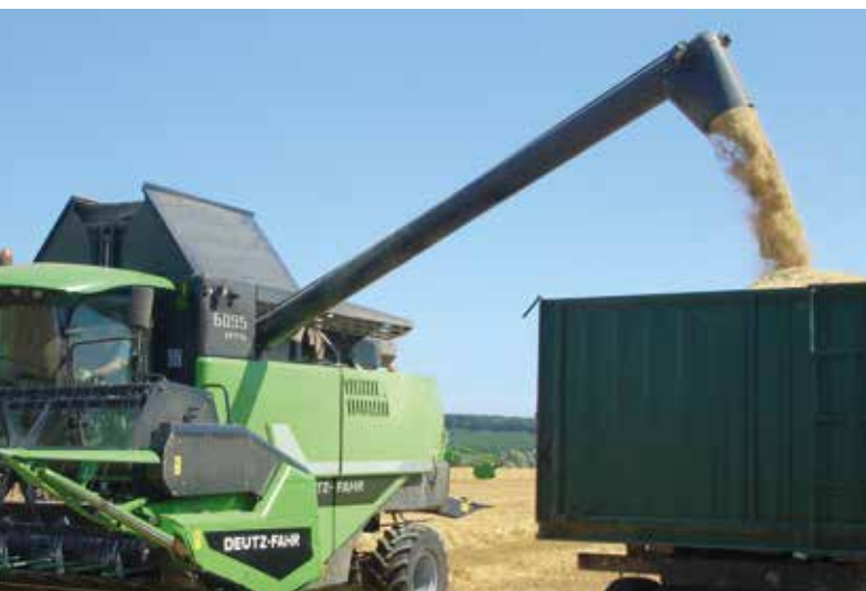
Grain unloading is made quicker and easier by the camera directed at the discharge pipe and an unloading speed of 90 l/sec.
