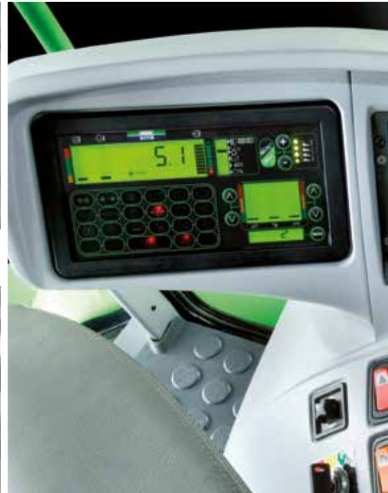
The new Combine Control Management system monitors performance of the machine in actual time.
