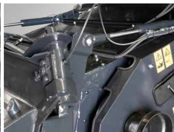
Electrohydraulic adjustment of the cutting angle ensures the position of the cutting bar is optimised relative to the direction of travel.
