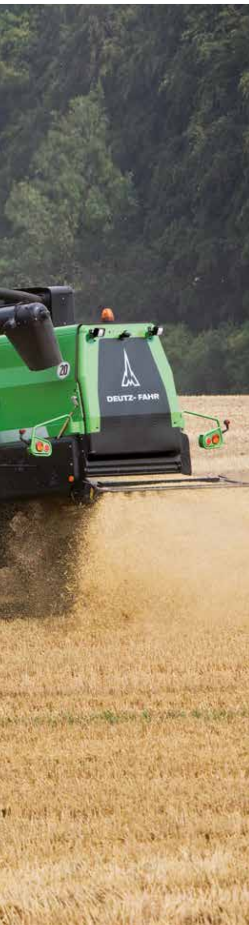
AUTOCONTROL adjusts the lateral and vertical movement of the header with notable precision, so as to maintain a steady cutting height and ensure that laid crops can be harvested to optimum effect, with the cleanest possible cut.
