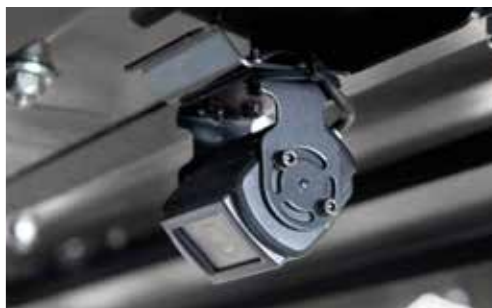
Rear camera directed at the towing hitch to facilitate hitching of the header transport trailer.
