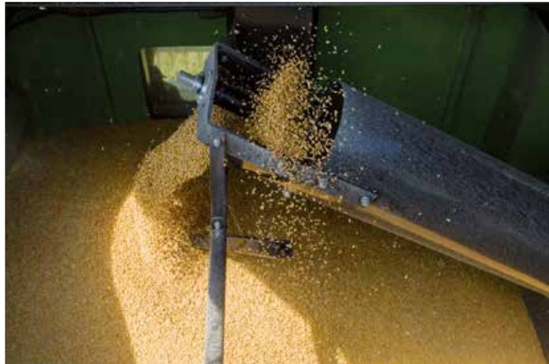
The folding coupling of the grain elevator greatly reduces the risk of crushing the grain."
