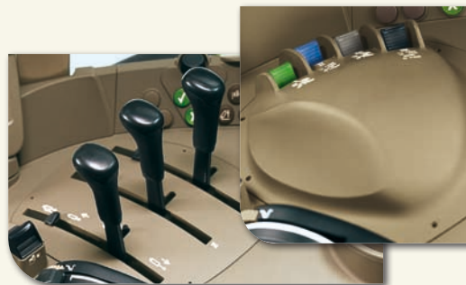
Choose M-SCV (left) or E-SCV (right) hydraulic controls. Both are positioned for quick use and precise implement adjustment.
