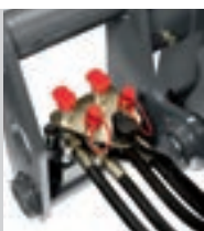
Two double-acting connections on the implement carrier
