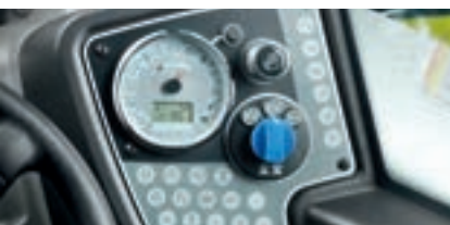
The selected speed range and the direction of travel are displayed on the instrument panel on the right.
