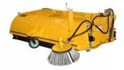
SWEEPER COLLECTOR Combined steel and polypropylene brushes tackle most material Generous hopper with hydraulic discharge operated from cab Heavy-duty one-piece canopy Gutter brush and dust suppression sprinkler options
