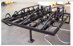
**BIG BALE TRIPLE GRAB** Easy handling of 3 × 800 bales or 2 × 1200 bales Curved tines penetrate and grip the bales without damage Hydraulically operated from the cab
