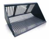
BEET BASKET Specialist attachment for handling all types of root crops Spaced bar design allows mud and small material to fall through Substantial toeplate gives long-lasting protection Round-bar leading edge to prevent damage to the crop Available with a choice of bracket options
