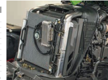
Additional fuel cooler for ideal power delivery.
