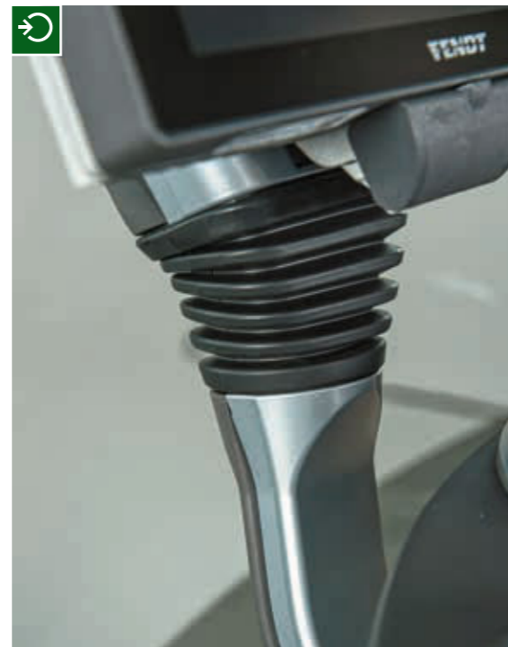
The Varioterminal can be adjusted in all directions thanks to a new bracket with a ball joint.
