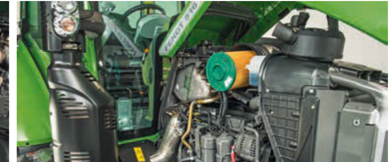
The air filter in the Fendt 500 Vario features a pre-separator for long filter service life and is easily accessible for maintenance works.
