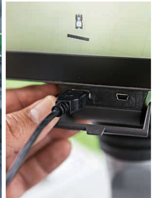
Field settings can be transferred to other Fendt tractors via the USB port. The port for charging mobile phones is also very practical.
