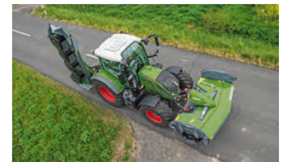
The Fendt 500 Vario reaches its final speed of 50 km/h at a low engine speed of only 1,700 rpm and 40 km/h at a mere 1,400 rpm.
