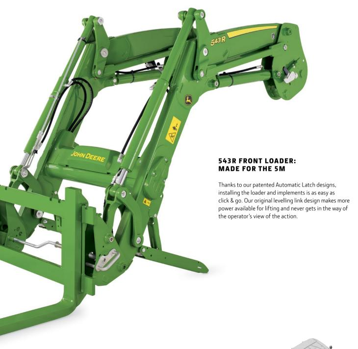
Quickly connect/disconnect implements as needed. Our patented auto latch system lets you automatically lock and unlock implements with the conveniently located release handle.
