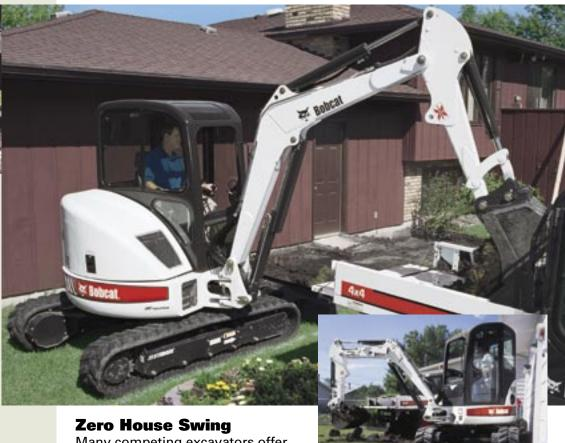
Many competing excavators offer Zero Tail Swing, but the 430 and 435 take the concept to the next level — **Zero House Swing** (ZHS). Not only does the rear of the machine stay within the excavator's width, so does the front end — the machine's left and right front corners! ZHS decreases the chances of accidentally striking buildings or trees during operation. And no damage to the machine or surrounding objects means lower operating costs!
